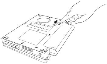
Sample battery release latch
